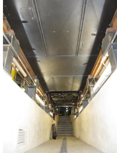
Figure 2: Underbody view of a typical low-floor streetcar, illustrating the lack of underbody equipment other than running gear.
